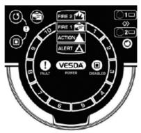
When the field service access door is open, the user has access to the RESET (5) DISABLE , Fire Test a , AutoLearn and Instant Fault Finder functions. When the Instant Fault Finder function is activated, the Smoke Dial converts to a fault indicator, with the dial segment numbers corresponding to the faults listed below.
